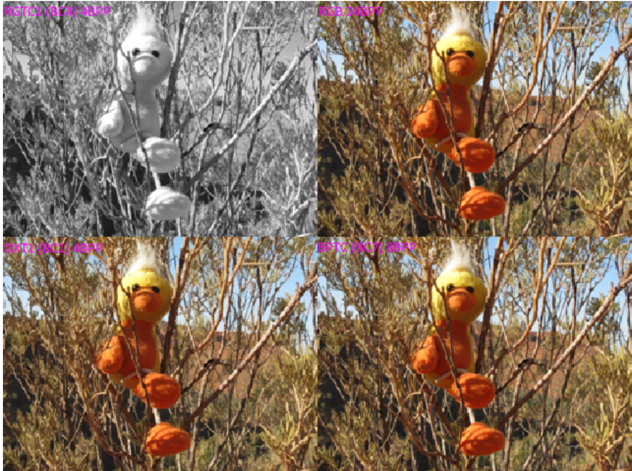
Four screenshots of the same image compressed in four different formats: RGTC1, RGB8, DXT1 and BPTC. Texture rendered with point sampling.
